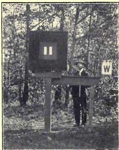
Fig. 2 —Background and Test Object used in determining effect of Stereoscopic Vision on discrimination of detail
