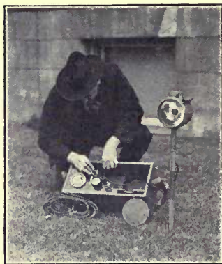
Fig. 7 —Trench Signalling Unit in operation
